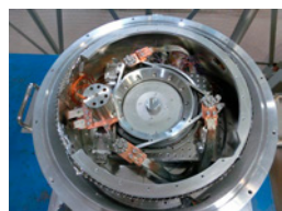
A rotary stage, which functions reliably at liquid nitrogen temperatures
