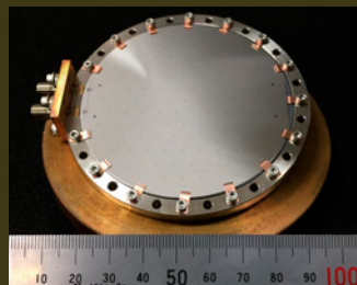
Microwave Kinetic Inductance Detectors (MKID) When millimeter-wave photons break superconducting Cooper pairs, the kinetic inductance and resistance in the superconducting transmission lines change. Based on this effect, MKIDs can use superconducting microwave resonators to detect millimeter-wave radiation.
